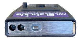
For locations where it is hard to read the meter's display, you can freeze the displayed number and then read it. Simply position the meter at the correct distance from the target and depress the pushbutton into the MEASUREMENT position. Depress again to the HOLD position to capture the measurement.
